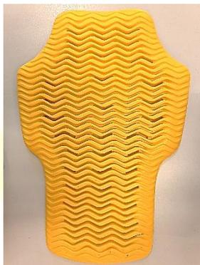
No fastening system is present, as the protector is designed to be inserted in special pockets of motorcyclists' clothing.
